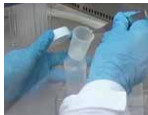
② Set Spheroid Catch into a 50ml centrifuge tube.
