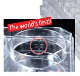
The outer scale on the wells allows for rough volume adjustments, reducing stress during works.
